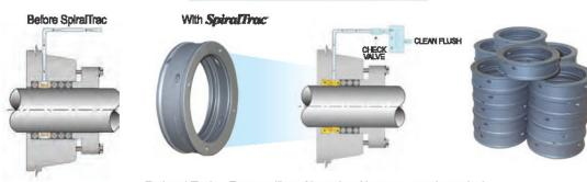
Reduced Flush · For use with packing only · No pump upgrade required
