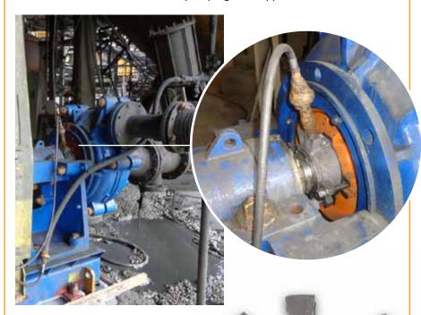
As a result customer is converting all concentrate pumps to Chesterton 442 split mechanical seals
